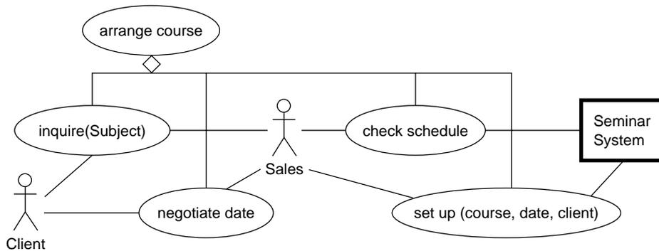
**Figure 1.15** Zooming in to the software system boundary.
