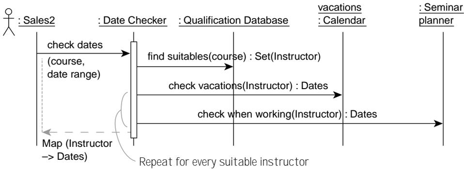
**Figure 1.23** Alternative sequence diagram, design version 2.
