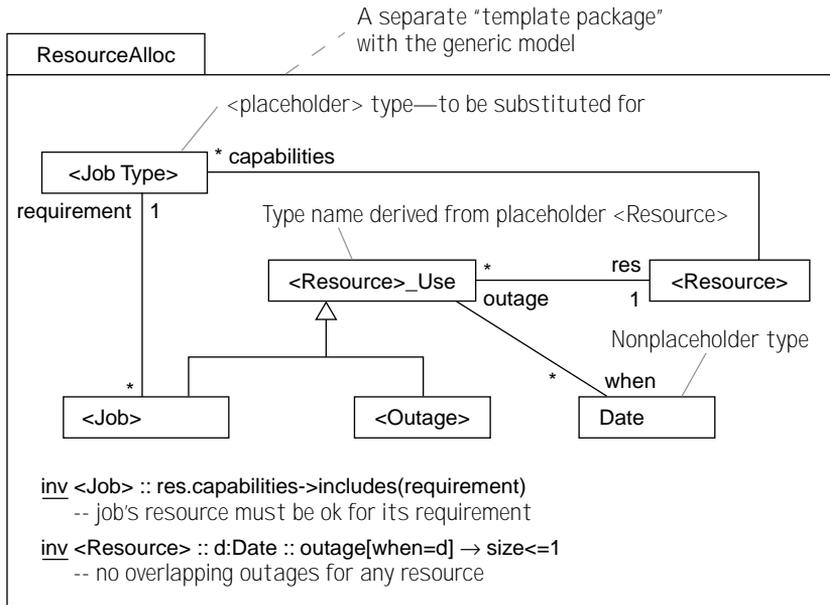
Figure 1.13 Generic framework model of resource allocation.
