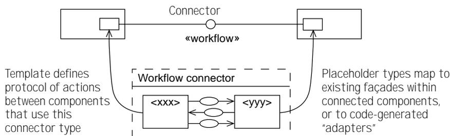
**Figure 1.33** Defining higher-level component connectors.
